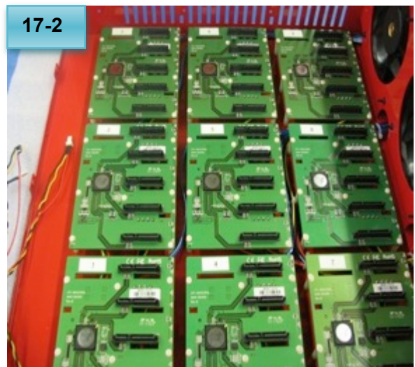
Connect and arrange the cables before installing the back plane.
